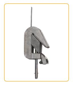
with test strip to determine absence of voltage Round Ø 5-35 mm Clamping range: Connection screw for earthing and short M12 circuiting cable: Cable cross section of the earthing and short circuiting cable: Max. 150 mm<sup>2</sup> Material (contact parts): - Strap: Aluminium alloy - Pressure piece: Aluminium alloy - Test strip: Galvanised steel Rated voltage/rated time/ 42 kA - 0.5 s - 2.5peak factor:
