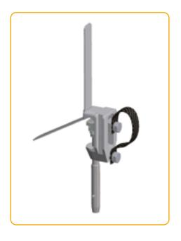
Contact wire: Ri 80-120 (DIN 43 141); Ø 10.6 - 13.2 mm Connection screw for earning and short circuiting cable: M10 Cable cross section of the earthing and short circuiting cable: Max. 50 mm<sup>2</sup> Material (contact parts): - Strap: Copper alloy, tin-plated - Pressure piece: Copper alloy, tin-plated - Test strip/catch device: Hot-dip galvanised steel Rated voltage/rated time/ peak factor: 14 kA - 0.5 s - 2.0
