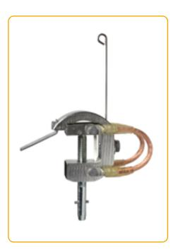
Clamp for contact wires Type Number 597 506 Model SNCB Contact wire: Single and double contact wire SNCB Connection screw for earning and short circuiting cable: M12 Cable cross section of the earthing and short circuiting Max. 50 mm<sup>2</sup> cable: Material (contact parts): - Strap: Copper alloy, tin-plated - Pressure piece: Copper alloy, tin-plated Stainless steel - Test strip: Hot-dip galvanised steel - catch device: Rated voltage/rated time/
