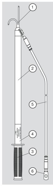
This one-polar device is a manually operated device for static discharge. The supplied device may differ from the picture in this instruction for use.
