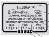
Marking of tools and equipment for live working
