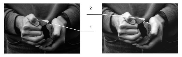
1. Hold the lower ring half (1) at the snap lock with one hand and strongly press on this ring half. At the same time pull on the upper ring half (2) with the other hand. When the snap-lock has opened up sufficiently the ring connector can be opened completely. This method is recommended for ring connectors that were <u>not</u> locked on the mains cable.
