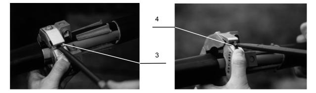
2. Insert a screw driver into the gap between the halves of the snap lock and carefully lever the lock open (3). At the same time press the lower ring half with the other hand (4) in order to open the gap between the ring halves further and this way facilitate opening the ring connector.
