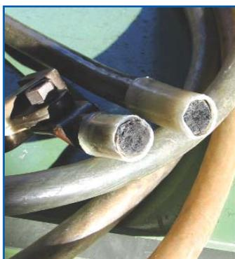
Standard DIN VDE 61230: 2009-07 (IEC 61230: 2008-07) in Annex C.3.2.2, Example 2, recommends to inspect earthing and short-circuiting cables for corrosion at least every five years (ten years for indoor use). The failure rate should be compiled and used to determine the frequency of inspection, related to usage and storage conditions.
