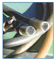
Standard DIN VDE 61230: 2009-07 (IEC 61230: 2008-07) in Annex C.3.2.2, Example 2, recommends to inspect earthing and short-cuiting cables for corrosion at least every five years (ten years for indoor use). The failure rate should be compiled and used to determine the frequency of inspection, related to usage and storage conditions.
