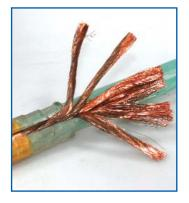
Reliability of devices serving primarily as security for persons must not be subjected to any compromise. For this reason those devices which are not clearly free of corrosion have to be withdrawn from further use.
