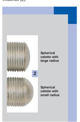
Spherical calottes with a small radius will easily penetrate the conductor as their contact area will grow slowly with each turn of screw, by which also the face pressure will only decrease slowly.
