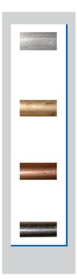
As material for contact screws different copper alloys have prevailed. Due to excellent electric conductivity, good machining properties, and unproblematic availability on the market they generally volunteer for electrically conductive parts.
