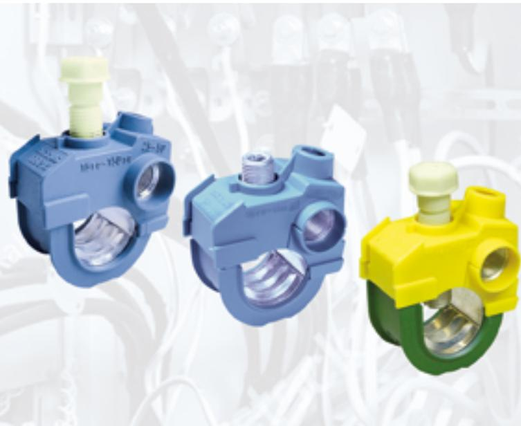
Insulation-piercing tap-off clamps are provided with insulation-piercing teeth, cutting edges or screws which spare removal of insulation from conductors.
