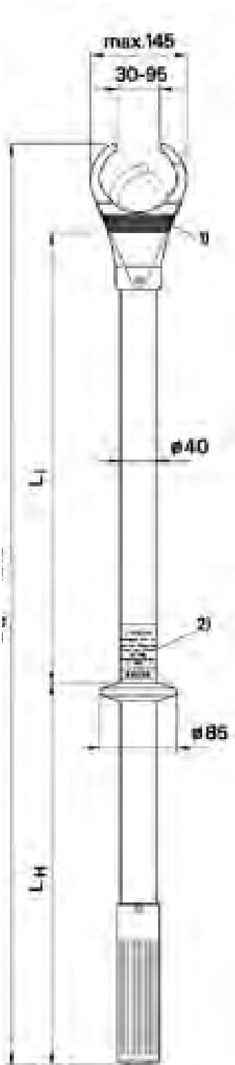
The fuse tong is used to grip an HRC-fuse from the front. By rotating the handle the HRC-fuse is held tightly by the clamping part. Little space is required by the fuse tong on each side. It is highly suitable for use in switching stations where space is limited.
