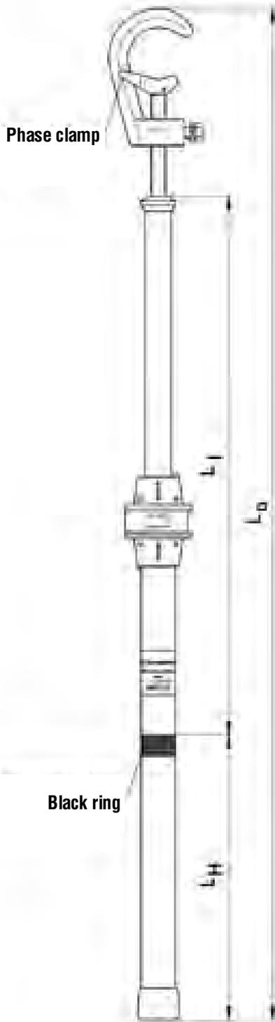
The length  $L_0$  of an earthing rod is mainly not determined by the insulating properties but by the condition to keep the operator at the necessary distance from live parts of the installation.
