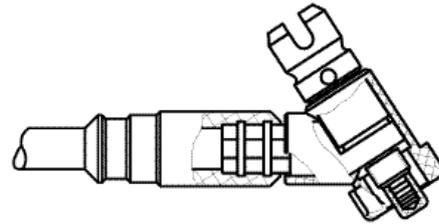
Fully insulated connection coupling
