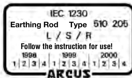
Fig. 2: Example of a label to IEC 1230
