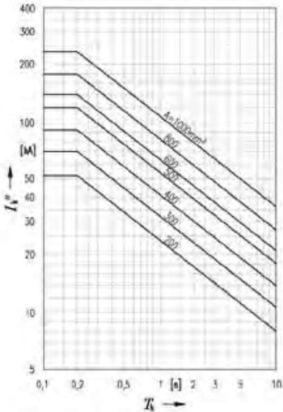
Fig. 4: Admissible current carrying capacity of short circuit bars made of pure aluminium E-Al F10
