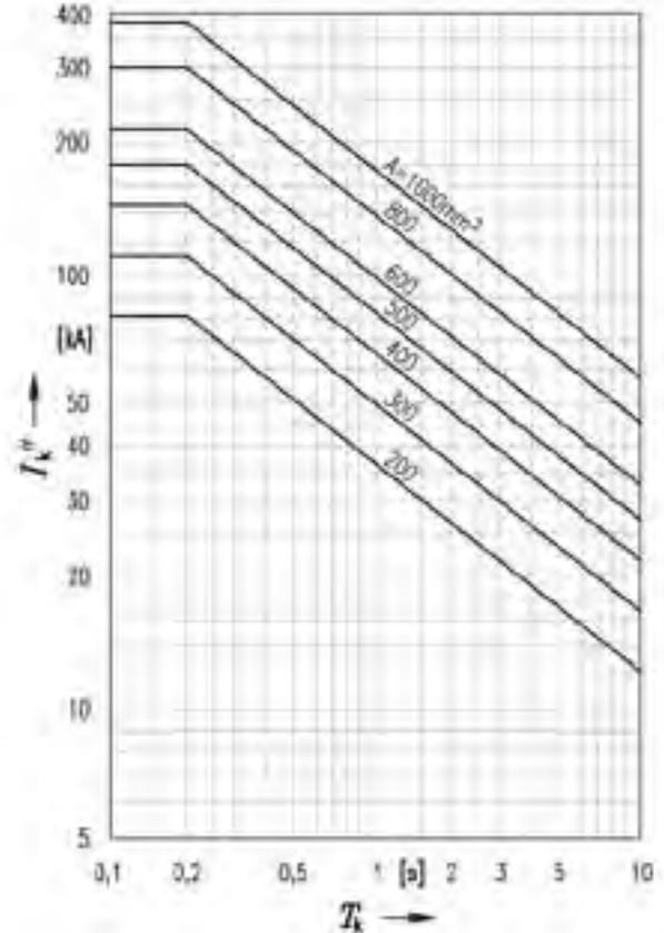
Fig. 5: Admissible current carrying capacity of short circuit bars made of electrolytic copper E-Cu 57 F20
