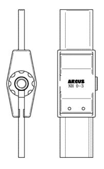
Plug-in blades made of red plastic material, metal part with threaded hole for torsion-safe connection to fullyinsulated connection coupling, fitted using the earthing handle (see page 18).
