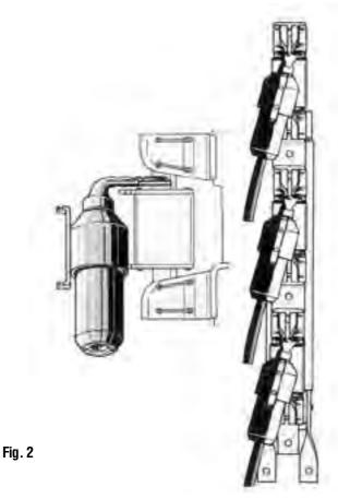
The plug-in cartridge consists of a fully insulated housing for a threaded fuse up to max. 63 A and an angular expanding contact with external spring. The cartridge is inserted to an operating DIN fuse by means of a commercially available DIN handle.
