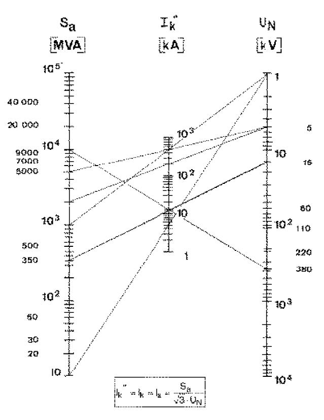
Fig. 6: Determination table short circuit current  ${\bf l_k}"$  of the mains breaking capacity  ${\bf S_a}$
