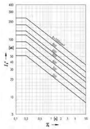
Fig. 4: Admissible current carrying capacity of short circuit bars made of pure aluminium E-AI F10
