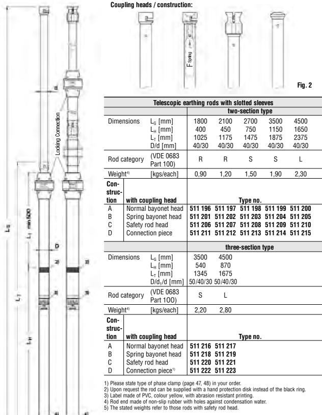
Material: Rods made of fibre glass reinforced epoxy resin, colour yellow, rod heads impact-resistant plastic material.
