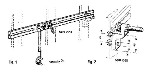
In the case of extremely high short circuit currents rigid short circuiting bus bars are of advantage. They offer simple assembly, little floor space and high resistance to short circuit strength.
