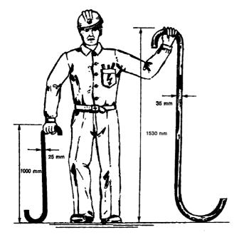
S-shaped hook for the rescue of persons from l.v. current circuits, working machines, etc., for example by: pulling on arms, legs, arm pits, neck or ankle, etc.
