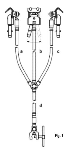
This device is equipped with the well-proven phase clamps made of tin-plated copper alloy with large contact surfaces, type 507 003. The swivel bayonet spindle is a particular advantage when mounting the clamp from an angular position.
