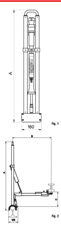
This device is used for short circuiting tracks with a lateral contact rail.
