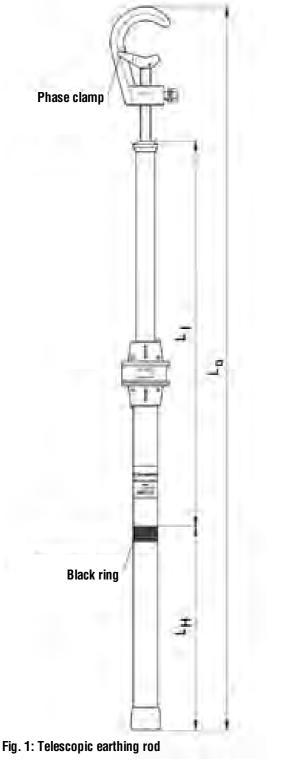
The length  $L_0$  of an earthing rod is mainly not determined by the insulating properties but by the condition to keep the operator at the necessary distance from live parts of the installation.
