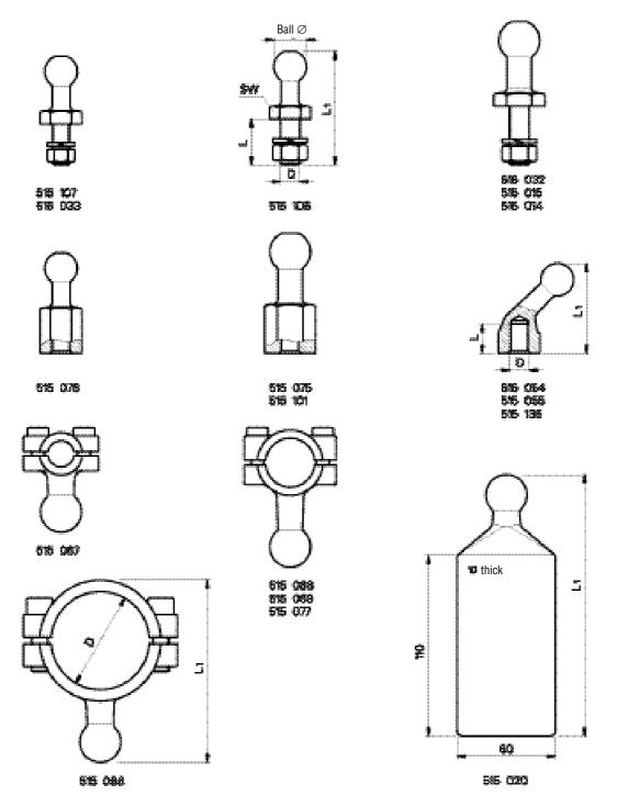
The spherical heads of the fixed points are manufactured with a very high-quality surface.
