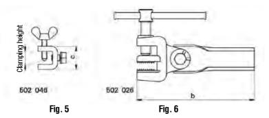
Clamp type 502 026 is tightened to the earth connection and by means of the handle it can be rotated at an angular range of appr.20 °, tightening the hand screw repeatedly. After the serrated contact surfaces have removed paint or other insulating layers on both sides of the earth connection the hand screw can be tightened completely.
