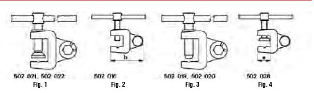
Notched clamps may also be used on tubular or round conductors.
