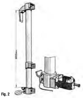
Fully insulated construction made of plastic material resistant to ultraviolet light, equipped with 2 clamps made of galvanized steel for cables up to 42 mm.
