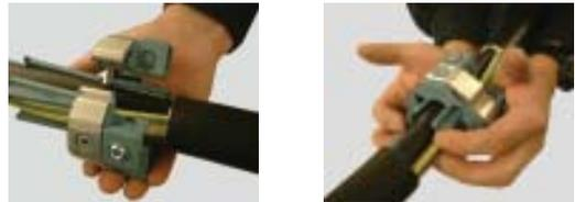
Installation of ring connector
