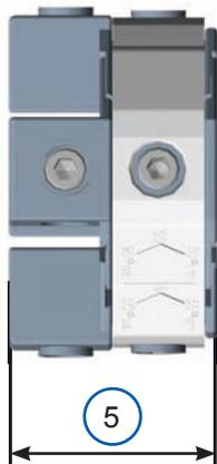
The ring connector width corresponds to the dimension of the ring connector expansion in direction of the mains cable. This dimension is relevant for selection of a suitable joint.
